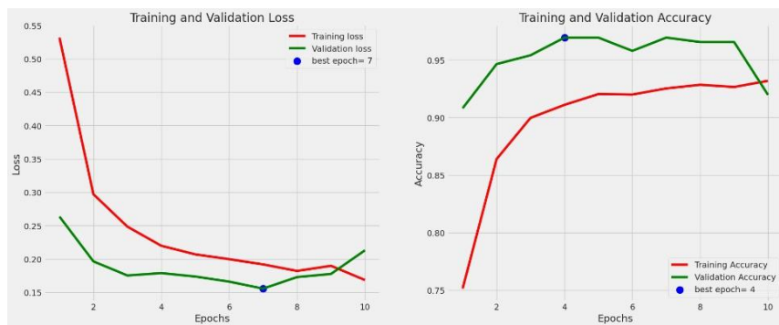
Image 2: Graph of the epoch and loss progression to achieve the best accuracy for the 2-layer convolution CNN architecture on the imbalance dataset
